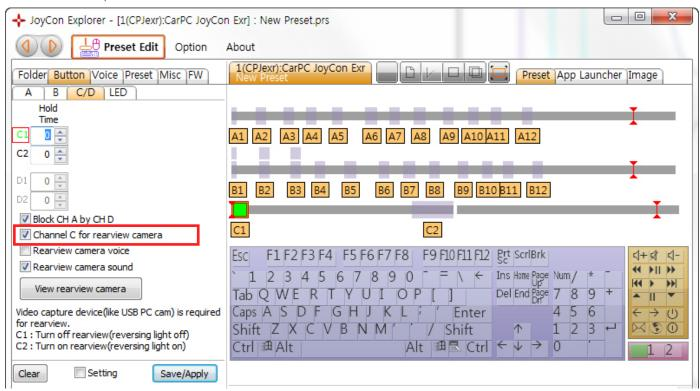
When you shift the gear lever to the reversing position, the reversing light is turned on and the reversing view pops up.
